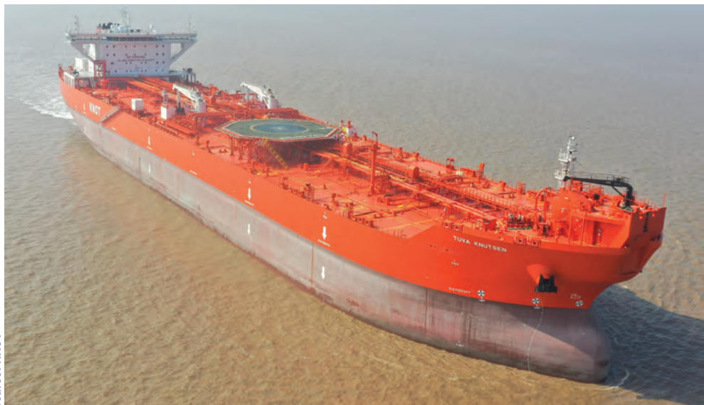
Knutsen NYK Offshore Tankers (KNOT) has multiple Suezmax-size shuttle tankers on order in China. The 152,700 dwt Tuva Knutsen is a Chinese-built unit of the fleet dating from 2021.
