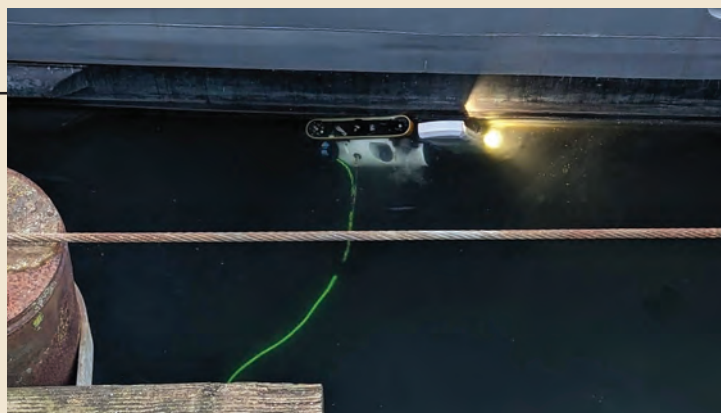
EverClean crawls the hull, capturing condition data tied to precise locations.
