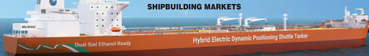
Digital rendering of a 154,000dwt shuttle tanker ordered by AET of Singapore and specified with ethanol-ready main propulsion plus a battery bank for peak shaving.
