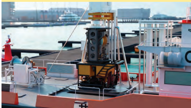
OceanAlpha's new 24-meter-class V180 USV-ROV system integrates a DP2-enabled offshore USV with a work-class ROV.
