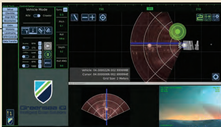
EverClean identifies an object on the hull and approaches for detailed inspection.
