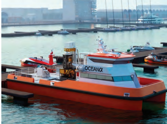
OceanAlpha's new 24-meter-class V180 USV-ROV system integrates a DP2-enabled offshore USV with a work-class ROV.
